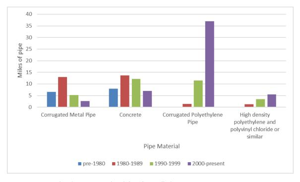
Figure 3-9 Lengths of pipe material and decade installed
