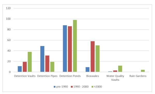
Figure 3-7 Types and numbers of stormwater treatment facilities in Sammamish and time period of installation
