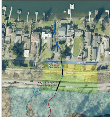
Zackuse Creek culvert replacement project and channel realignment at East Lake Sammamish Parkway
