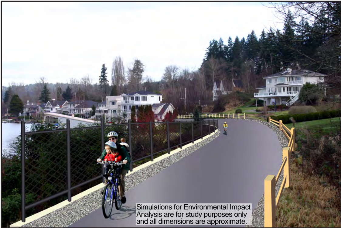
Corridor Alternative; Looking north from railbed in north-end Sammamish Place neighborhood. Paved path is 12 ft. wide with 3 ft. shoulder on left and 2 ft. gravel shoulder on right.
